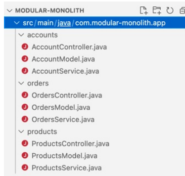
Figure 27: This Java monolith has been split into independent modules.
