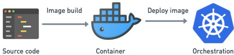
Figure 24: Containerizing your monolith is a way of standardizing deployment, and it is an excellent first step in learning Kubernetes.
